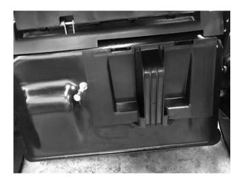
To use the back discharge function, you must open the back flap of the tool. Insert the mulching adapter on the hole on the back. Release the flap.
